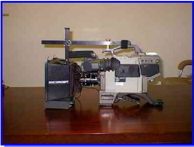
Photo of the Classic Microprompt rigging showing mounting on the carrying handle.
