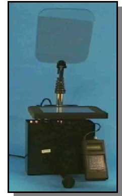
Fastpole fully closed. Glass can be programmed to come to rest horizontally).
